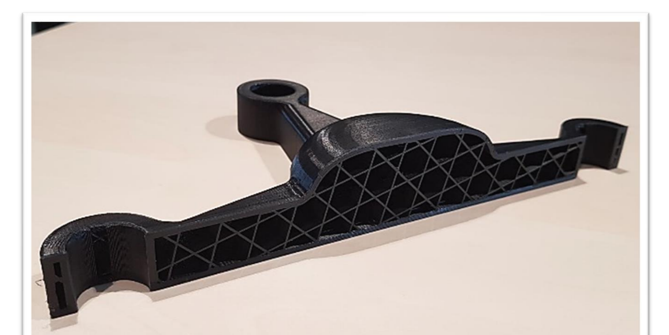
3D-printed mock-up of fibre-reinforced body
