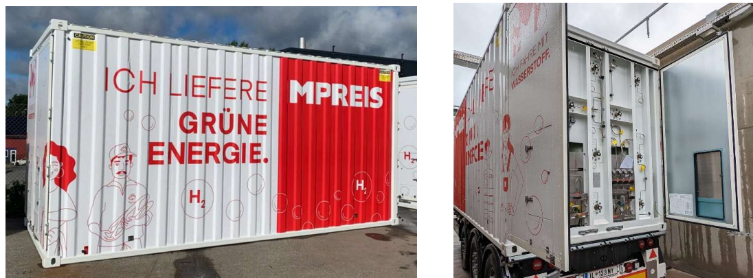
Figure 9. 20-foot hydrogen MEGC from MPREIS, with permission from MPREIS.
